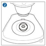
Put a specimen on the stage plate.
